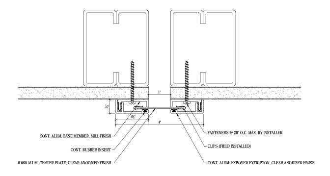
NOTE: 1 HOUR CONSTRUCTION INDICATED 2 LAYERS OF GYPSUM BOARD FOR 2 HOUR CONSTRUCTION
